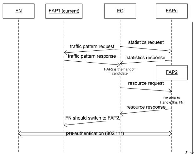
Figure 4. Sequence of messages in the handover procedure.
